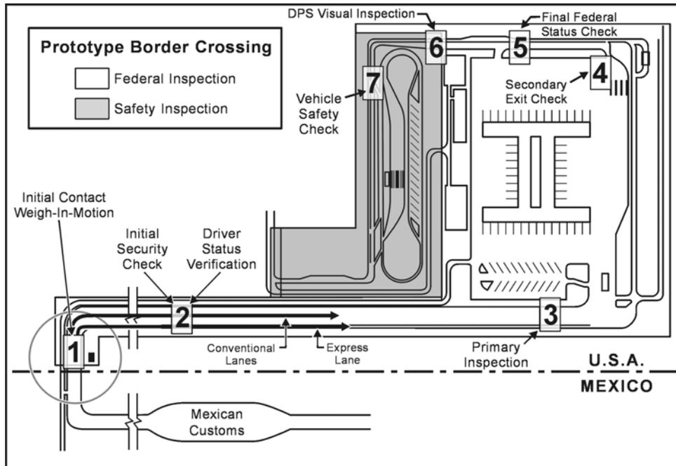
**1** Initial contact with the vehicle is made at the station, the **vehicle is identified** and its **electronic file activated**, the vehicle is weighed by a **weigh-in-motion** system. If overweight the file is flagged for further processing by appropriate agencies. (Ideally, this station would be upstream of the Mexican export station to screen out overloaded vehicles before they cross the border.)
