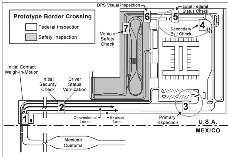
**4** At the exit from the **secondary** (detailed) inspection area, the status of all inspections is checked electronically at this station. The vehicle is tracked to ensure compliance and if it has not been cleared to exit, signing at Station 4 will instruct the driver to return for further processing. This station will ensure that vehicles routed into the secondary inspection area have had their record cleared by those inspectors sent to examine that vehicle.
